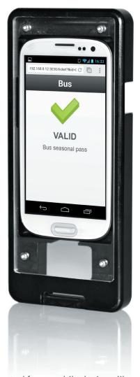
NFC Eye is a system for access control from mobile devices, like smartphones and tablets, equipped with the NFC (Near Field Communication) technology. Thanks to its user-friendliness and limited costs, NFC Eye is the ideal solution for access control with the aid of an operator in car parks, on means of transport, or during parties or events where fixed reading devices cannot be installed.
